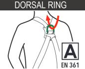
The rings marked with "A" are the only attachment points that can be used for arresting a fall! Only to these points it is allowed to connect one of the following fall arrest equipment:
